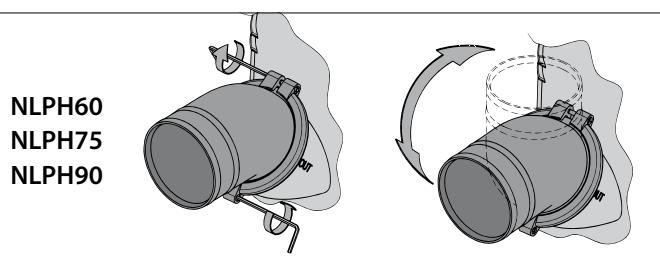
Loosen the bolts before turning the hose connections!
