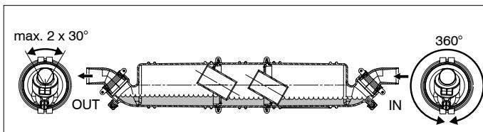
For a proper working it is essential that the OUT half of the housing and the inner part placed within this are in the relative positions as shown in the illustration. A deviation of maximum 30° to either side is permitted.
