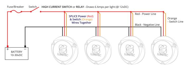
NOTE: The SBX2 can also be wired in a standard two wire installation as well by simply connecting the red and orange wires together and powering via an appropriately rated switched power bus.
